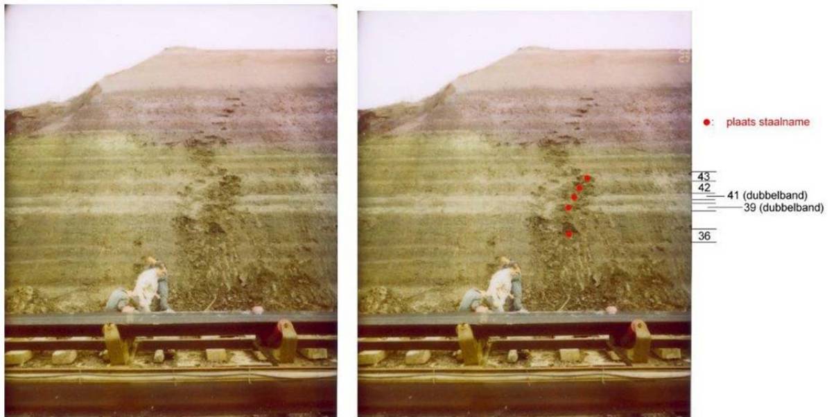
Figure 5 – Sampling for hydraulic conductivity in the Putte Member (Terhagen, Rumst).
