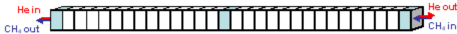
Figure 3: Geometry used in the diffusive transport model. Blue cells indicate where the evolution of the dissolved gas concentrations is recorded.
