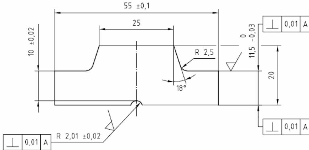
Figure 1 – Support block for the static calibration of instrumented strikers recommended by ISO 14556:2000.
