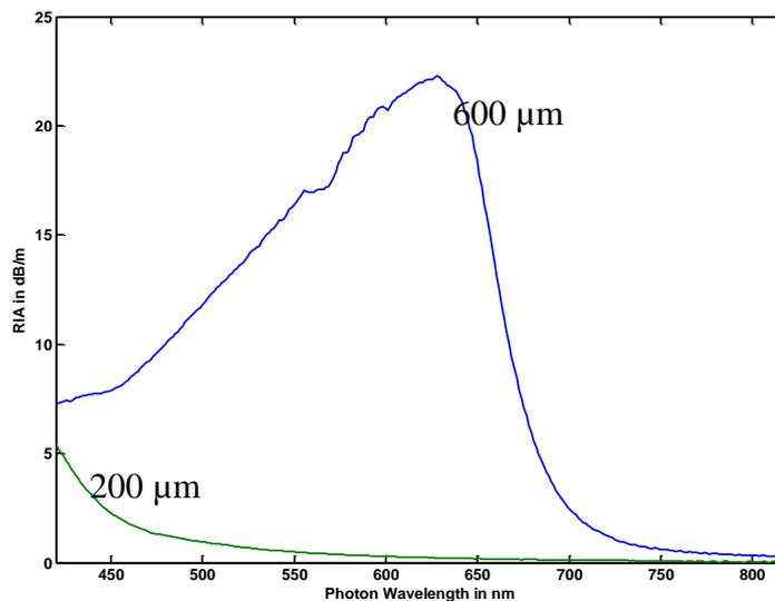
**Fig 2: Comparison of the RIA in 600 μm SSU and 200 μm STU Al-coated pure silica core fibres loaded with hydrogen at the same time and irradiated simultaneously at  $1.610^{16}$  n/cm<sup>2</sup> ( $E>0.1$ MeV) and 2 MGy.**
