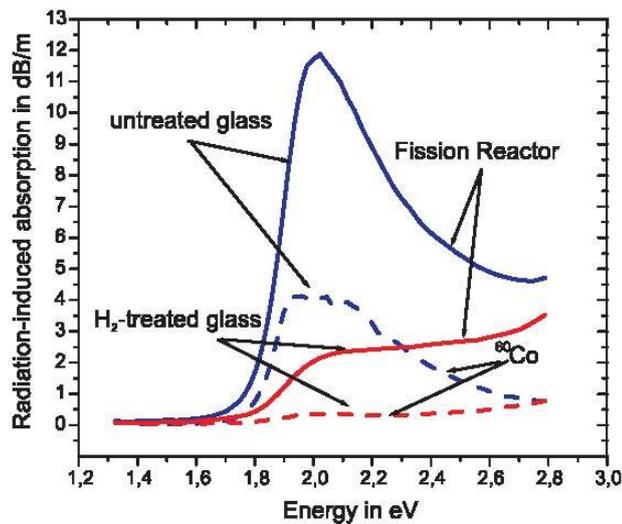
Fig 4: Spectral comparison of the RIA in the KU1 and KU1+H2 (KU2) fibres following a  $^{60}\text{Co}$  irradiation up to 3 MGy or a fission reactor irradiation at the same ionising dose and about  $2 \times 10^{17} \text{ n/cm}^2$  ( $E > 0.1 \text{ MeV}$ ) [6].
