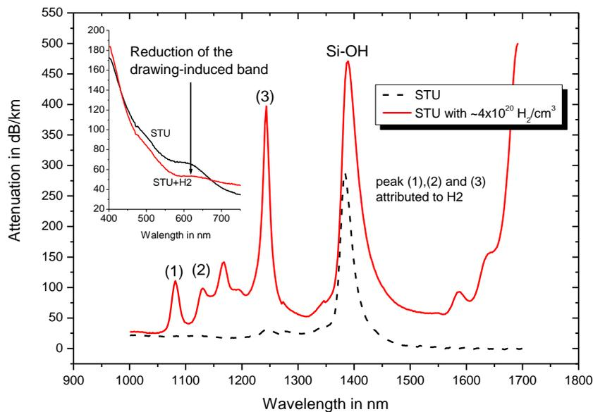
**Fig. 1- Comparison of Infrared-optical attenuation spectra of H<sub>2</sub>-treated and untreated low-OH unirradiated silica fibre. The inset shows the reduction of the drawing induced band due to the action of H<sub>2</sub>.**
