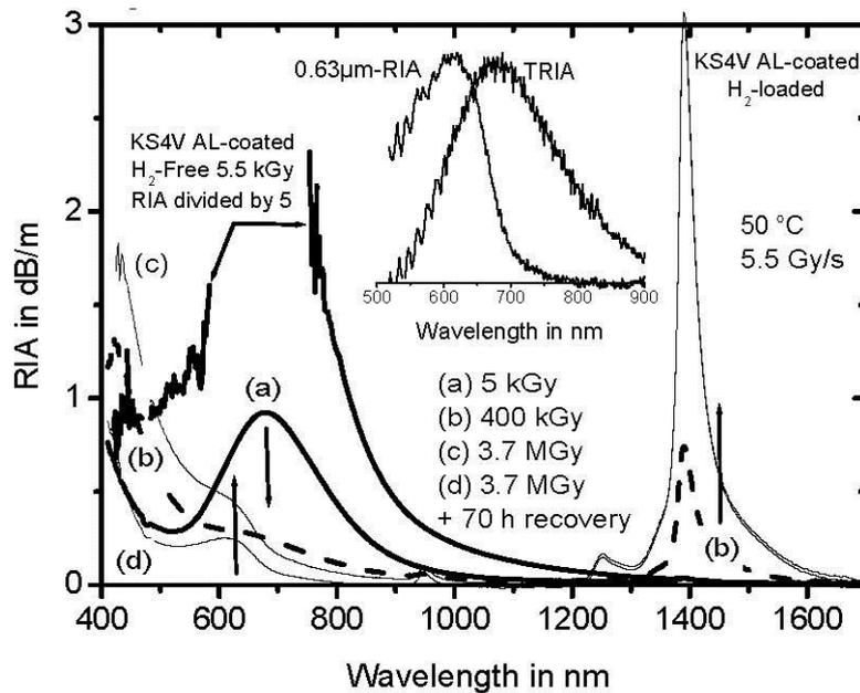
Fig 2: Decrease in the Transient RIA (TRIA) at 700 nm followed by the RIA increase at 630 nm as a function of the dose in  $\text{H}_2$  treated aluminium-coated fibres. For comparison the corresponding TRIA in  $\text{H}_2$ -free aluminium coated KS4V fibre is also shown with a reduced factor of 5. The inset compares the shape of the TRIA and 0.63  $\mu\text{m}$ -RIA in normalized axis when influence of the UV tail is removed.
