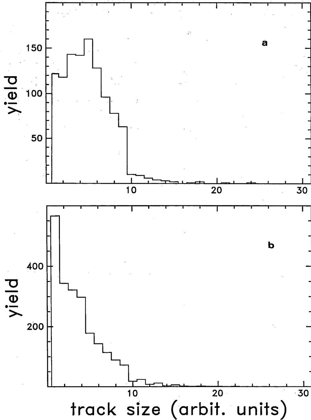
**Fig. 5:** In part (a) a characteristic track area-distribution is shown consisting of two components. In part (b) the respective distribution for detector (4) from run (1) is displayed showing a strong enhanced component of small areas due to a higher contribution of high energy  $\alpha$ - particles from  $^{214}\text{Po}$  (see text).
