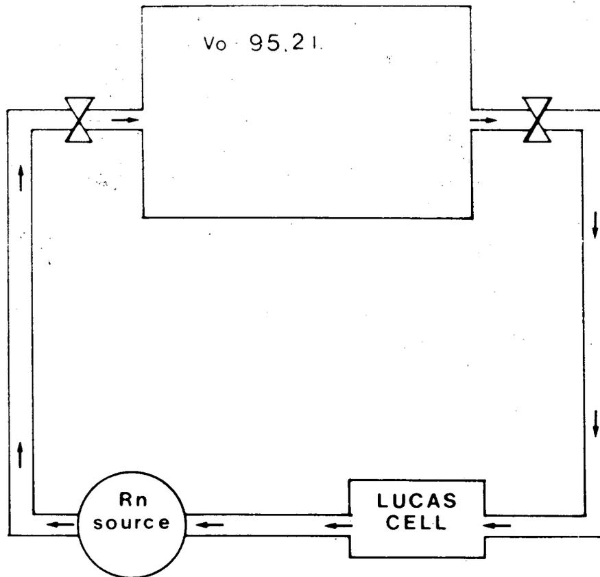
**Fig. 2:** Experimental setup used in the calibration phase of the personal radon dosimeter.
