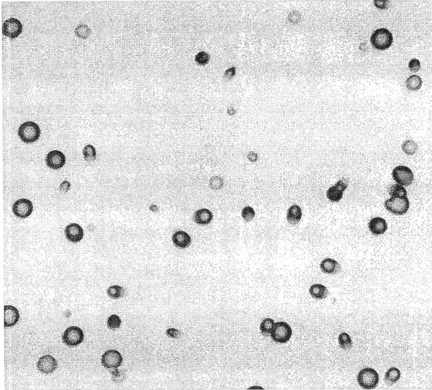
**Fig. 3:** Example for etched  $\alpha$ - particle tracks in CR-39 material. The size of the tracks depends on the  $\alpha$ - particle energy. The shape of a track becomes more excentric with an incident angle deviating from being perpendicular to the surface (the height and width of the image is 0.562 mm and 0.612 mm, respectively).
