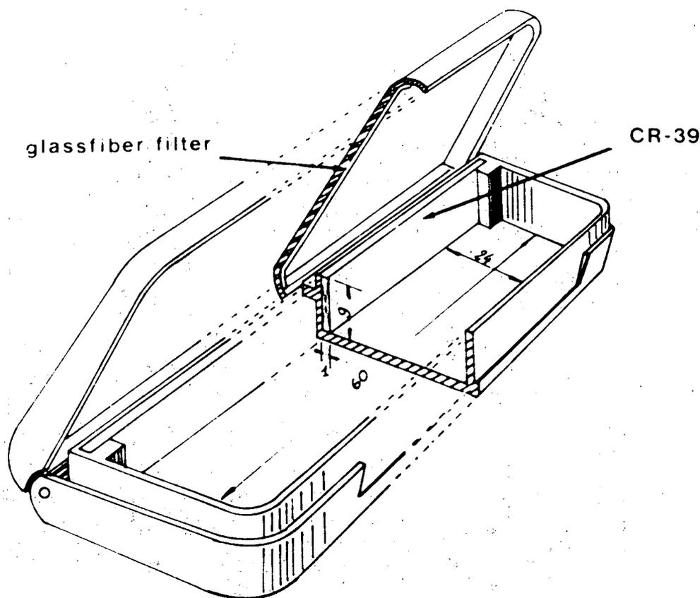
Fig. 1: Schematic representation of the personal radon dosimeter (all measures are in mm). The CR-39 detector is placed on the backside of the dosimeter.
