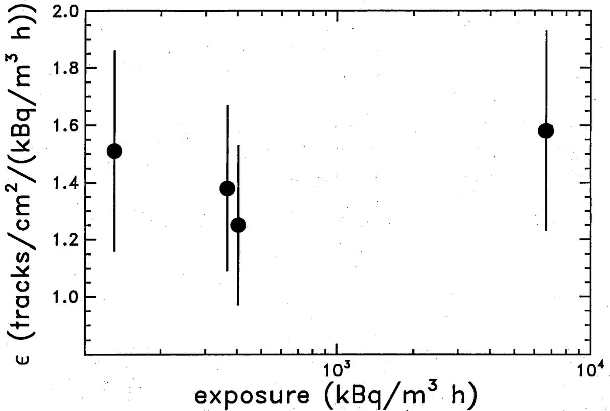
Fig. 6: Efficiency of the personal radon dosimeter as a function of the radon exposure for image processing based track-counting.
