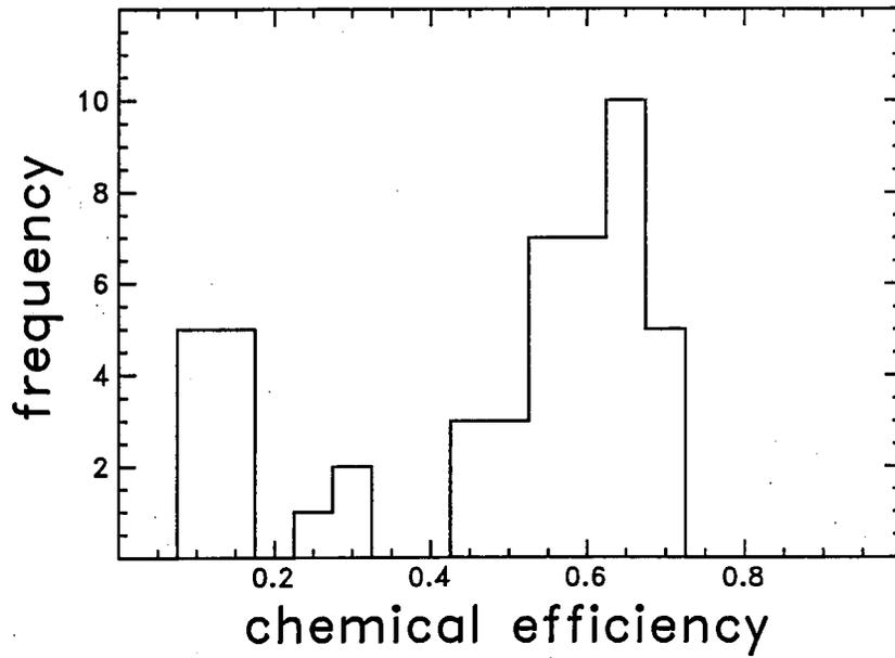
Fig. 4: Frequency distribution of the efficiency of the chemical separation of  $^{210}\text{Po}$  deposited in polyester material.
