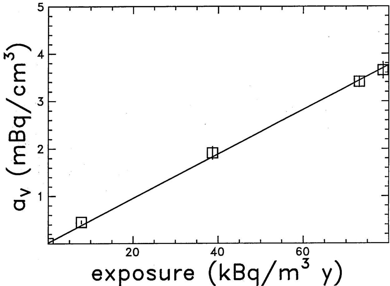
Fig. 6: Volume activity  $a_v$  as a function of the radon exposure. The full line gives the result of a linear fit to the data. The relative uncertainty on the fitted slope is 1.9 %.
