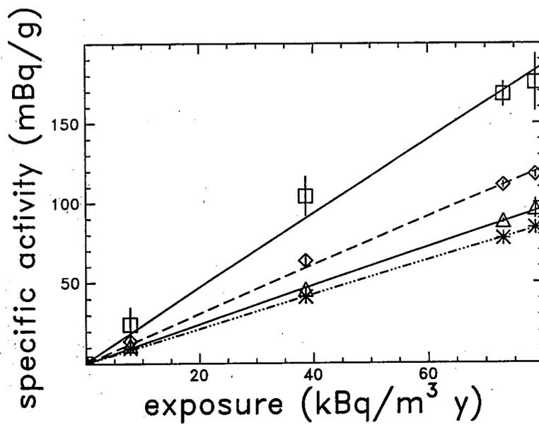
Fig. 5: Specific sample activity  $a_s$  as a function of the radon exposure. Different symbols refer to different sample densities. The order is according to Tab. 2. The lines indicate the respective fit to the experimental data.
