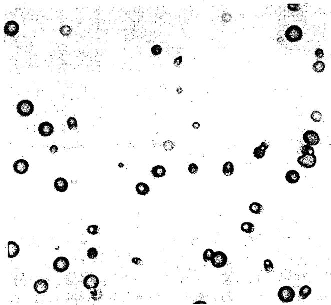
**Fig. 2:** Example of etched  $\alpha$ - particle tracks in CR-39 material. The size of the tracks is of the order of  $\mu\text{m}$  and depends on the  $\alpha$ - particle energy. The shape of a track depends on the incident angle of the  $\alpha$ - particle on the detector's surface.
