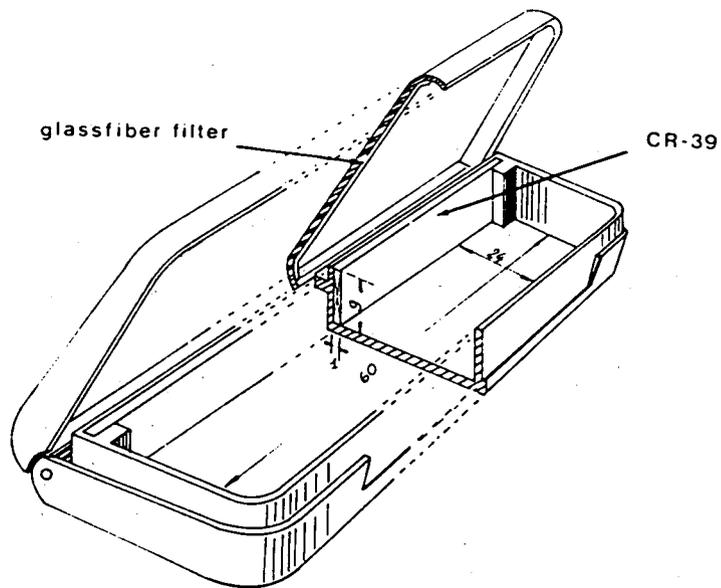
**Fig. 1:** Schematic representation of the SCK•CEN personal radon dosimeter (all measures in mm)
