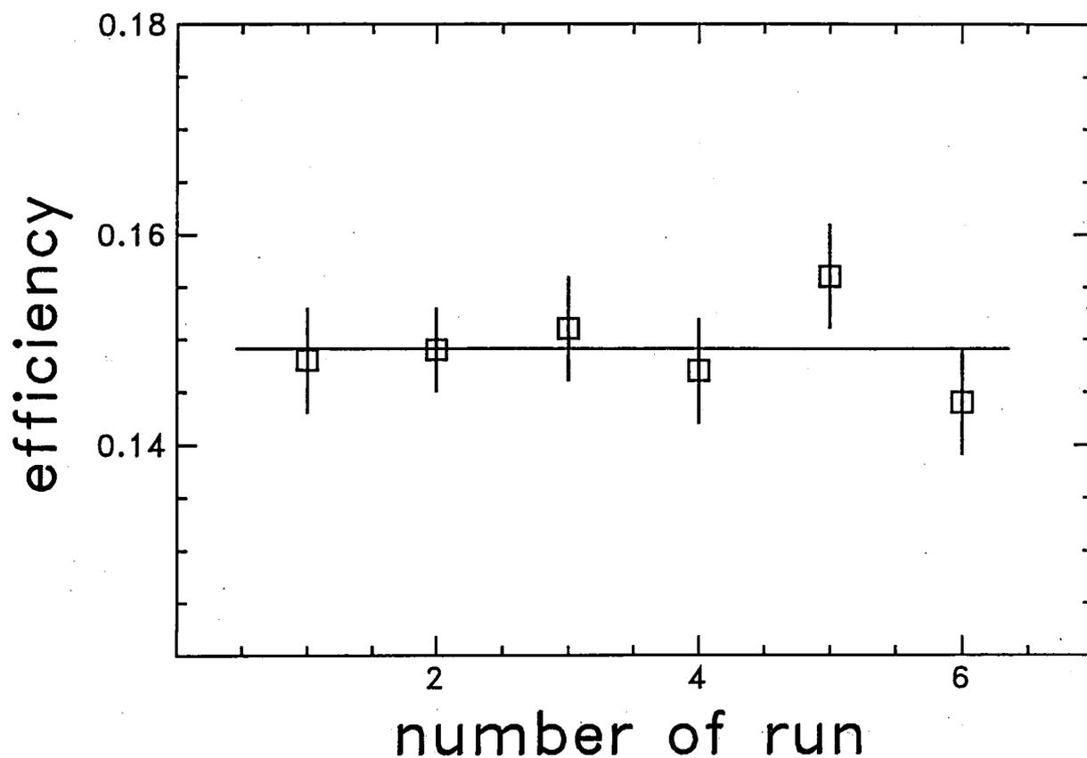
Fig. 2: Efficiency of sampling channel (1) obtained at a distance of 0.7 cm from the detector. The full line indicates the weighted average of the data.
