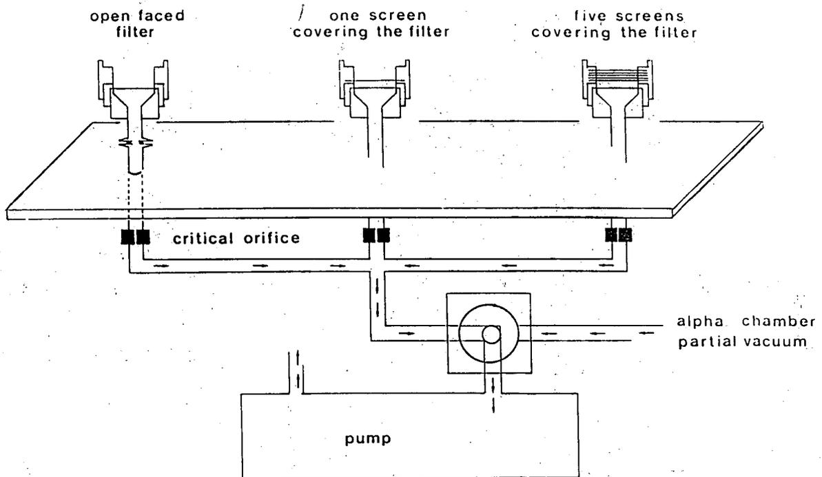
Fig. 1: Sampling section of the bronchial dosimeter. The open diameter of one sampling channel is 4 cm. The flow rate at standard atmospheric conditions is 9.1 l/min leading to a face velocity of 12 cm/s.
