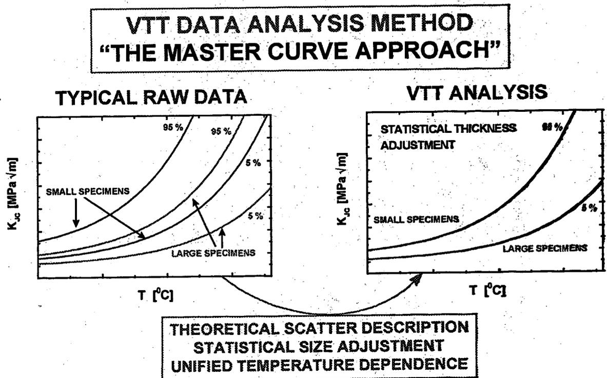
Fig. 1 Principle of the Master curve method.
