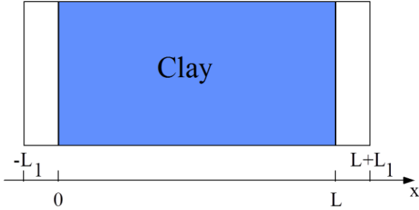
Figure 3: Configuration of the through diffusion model
