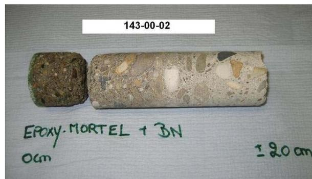
Figure 22: Concrete core of hot spot N°2 in room 143
