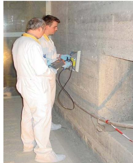
*Figure 4: Measurement using a “Seletra”, a hand-held plastic scintillator*
