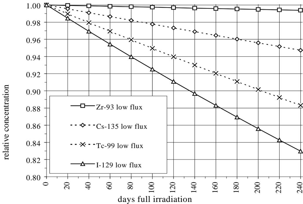
Figure 5 Evolution of selected LLFPs in high thermal flux positions in Myrrha, with  $v_0 \int_0^{0.5} n(E) dE = 3.0 \times 10^{15} \text{ n/cm}^2 \cdot \text{s}$
