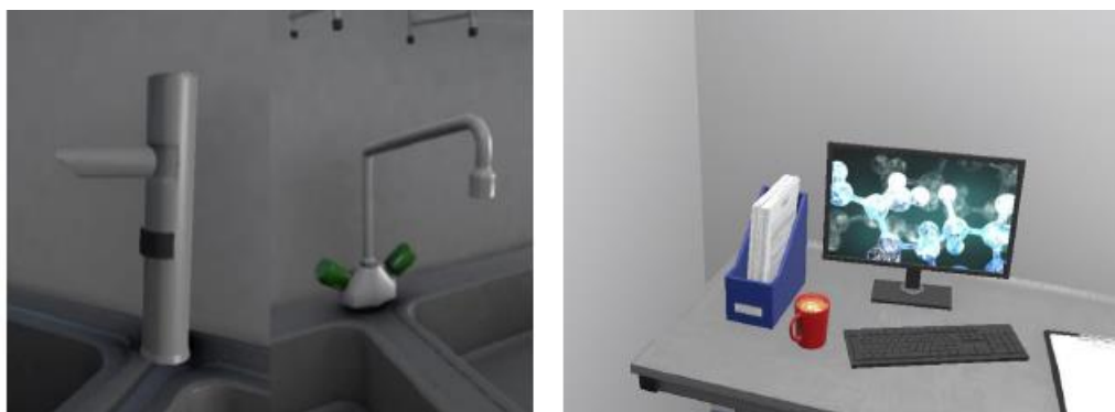
Figure 3 left: Comparison of contact-free water tap recommended for RC2 and obligatory for RC3 and usual water tap. Right: A cup of coffee in the laboratory as example for an obvious error.
