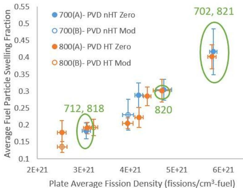
Fig. 1. Plate-average swelling fraction vs fission density for the 700 and 800 series plates irradiated in EMPIrE. The circled and numbered plates are those with available DE.
