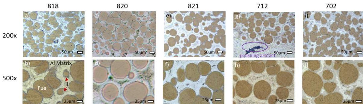
Fig. 2. Selection of micrographs from plates 818 (a&b), 820 (c&d), 821 (e&f), 712 (g&h), and 702 (i&j) at 200x and 500x magnifications. U-7Mo fuel is the dark phase, the Al matrix is the brightest phase, and the interaction layer is medium grey, as exemplified in image b.
