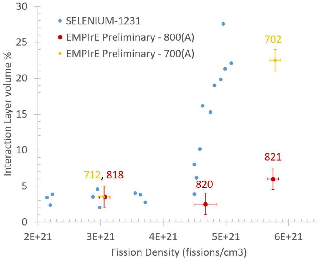
Fig. 3. Preliminary EMPIrE IL volume % compared to SELENIUM-1231. The y-axis error bars in the figure indicate the data variance.
