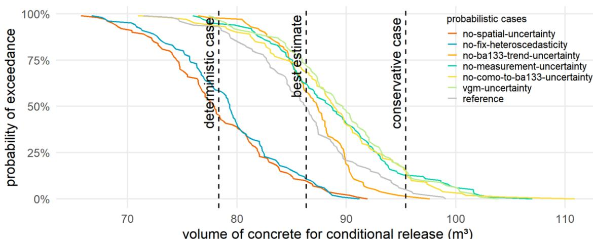
**Figure 4: Complementary cumulative distribution function for the volume categorized as conditional release, in function of the different cases with respect to uncertainties**
