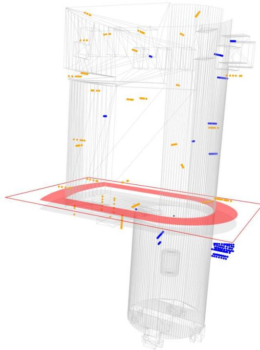
Figure 5: 3D representation of the BR3 biological shield showing the location of one of the horizontal cross sections. Markings in blue and yellow represent different sample locations
