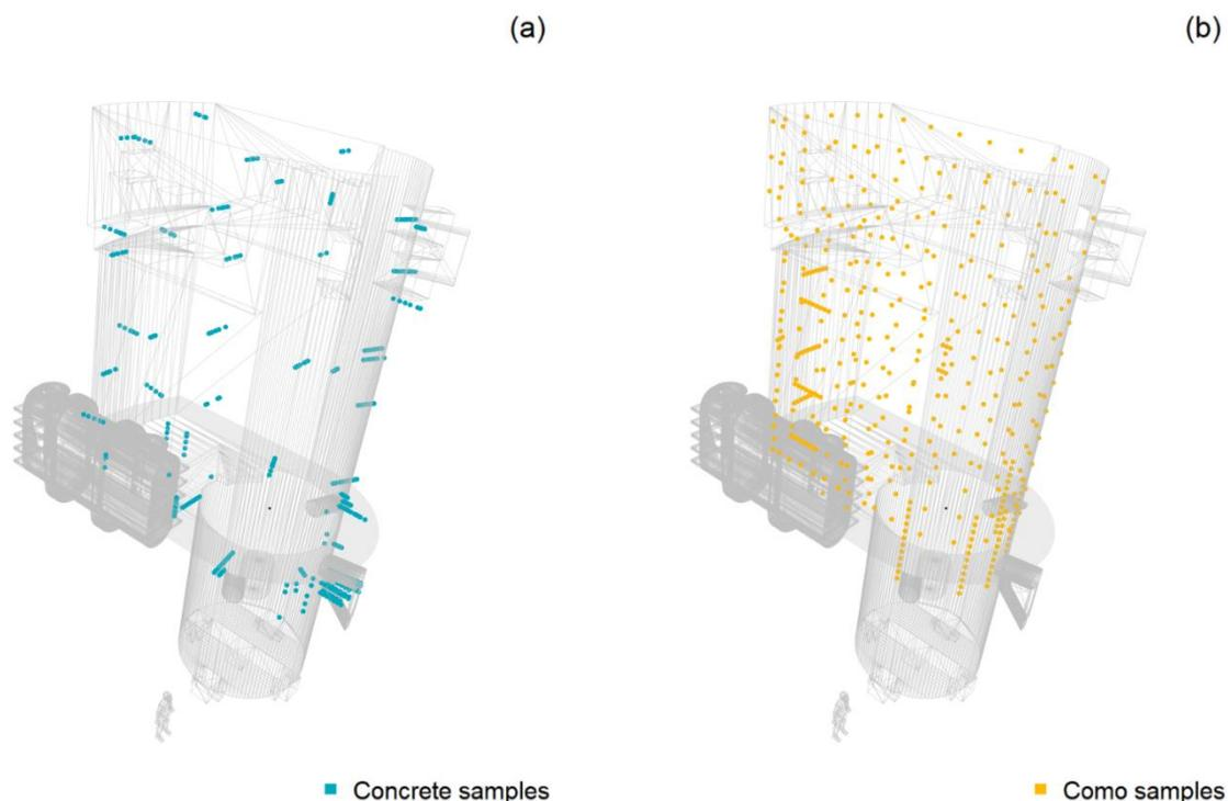
**Figure 3: Overview of the borehole (a) and in-situ total gamma (b) data locations used for the final dataset. Como samples refers to the use of the COMO300G (Nuvia) handheld device used for the measurements.**
