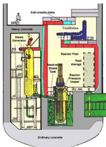
**Figure 1: Cross section of the BR3 reactor building during exploitation showing the main components. The building structure is mainly composed of reinforced ordinary concrete (bottom plate) and reinforced heavy concrete (upper structure). The activated concrete is marked in red colour (first rough estimation).**
