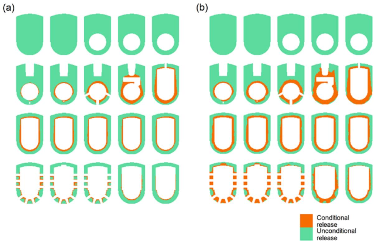
Figure 6: Selection of horizontal sections of the biological shield for different heights. On the left (a) we show the best estimate categorisation (median of the reference case), while the right figure (b) shows the conservative estimate categorisation (95th percentile of the reference case).
