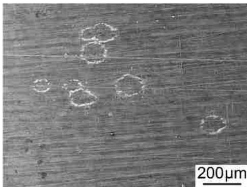
Fig. 7. Secondary-electron image of surface area populated with pits on Fe-14Cr-2Mn-20Ni-0.5Cu-3Al sample after the test at 500 °C in static Pb-Bi eutectic for 10,000 h. Sample is cleaned chemically with respect to solidified Pb-Bi.
