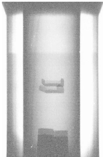
*Fig.13.2 is an X-ray picture of the balance pan. The picture is a double exposure, one of the tray at room temperature and one at liquid nitrogen. The film, on the outside of the Dewar tail, remained at room temperature. Cooling causes the shrinking of the copper wires that suspend the sample holder, lifting the latter.*
